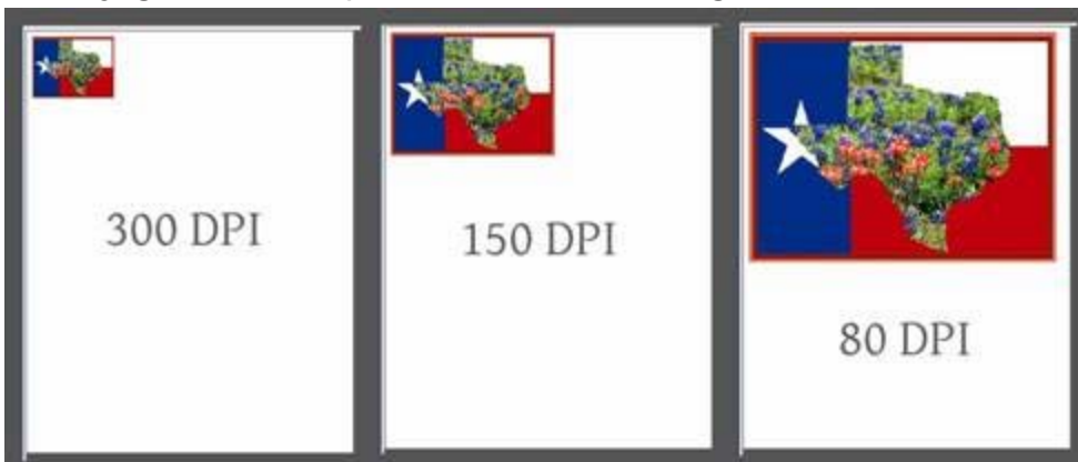
Figure 3 (above) The exact same picture printed at 3 different DPI's. Dithering is the use of somewhat randomized scattered dots. This tends to look smoother than grids, but the theory is similar. One image pixel can require several printer dots.
